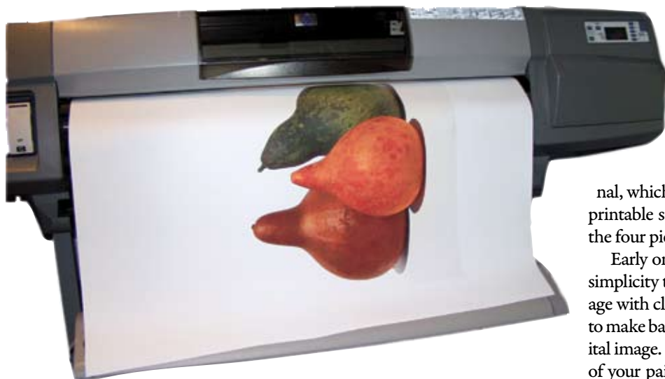
The first print coming off of my 42-inch HP Designjet 5000 PS UV. Note the extra space around the image to allow for stretching.
